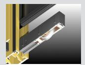
The key to making high performance sliding windows is to use large diameter, high performance wheels. We use sliding door wheels in the 602 and when the panels are double glazed or extra heavy, we use double bogey wheels.
